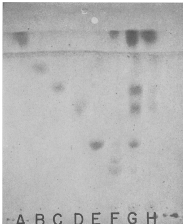
FIG. 4. Photograph of a chromatogram showing the separation of phosphatides on glass paper impregnated with 2% sodium silicate solution. Developing solvents: First, benzene, developed to upper front (14 cm.). Second, benzene-pyridine-water (BPW 100-125-13, developed until solvent traveled 5 cm., then transferred directly to third solvent. Third, BPW 100:125:25 until solvent rose to lower front (12 cm.). A. Triglyceride and cholesterol. B. Fatty acid. C. Phosphatidyl choline. D. Sphingomyelin. E. Phosphatidyl ethanolamine (PE) F. Mixture containing (in order of decreasing R_f ) neutral lipid, PE, lyso-PE and phosphatidyl serine. G. A chloroform-methanol extract of blood serum.
