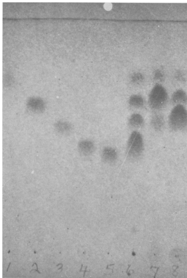
Fig. 2. Photograph of a chromatogram showing the separation of methyl esters on "silica gel" paper. Developing solution: Isooctane. 1. Methyl stearate and palmitate. 2. Methyl oleate. 3. Methyl linoleate. 4. Methyl linolenate. 5. Methyl arachidonate. 6. Mixture of 1, 2, 3, 4, and 5. 7. Methyl esters of vegetable shortening. 8. Methyl esters of cottonseed oil.
